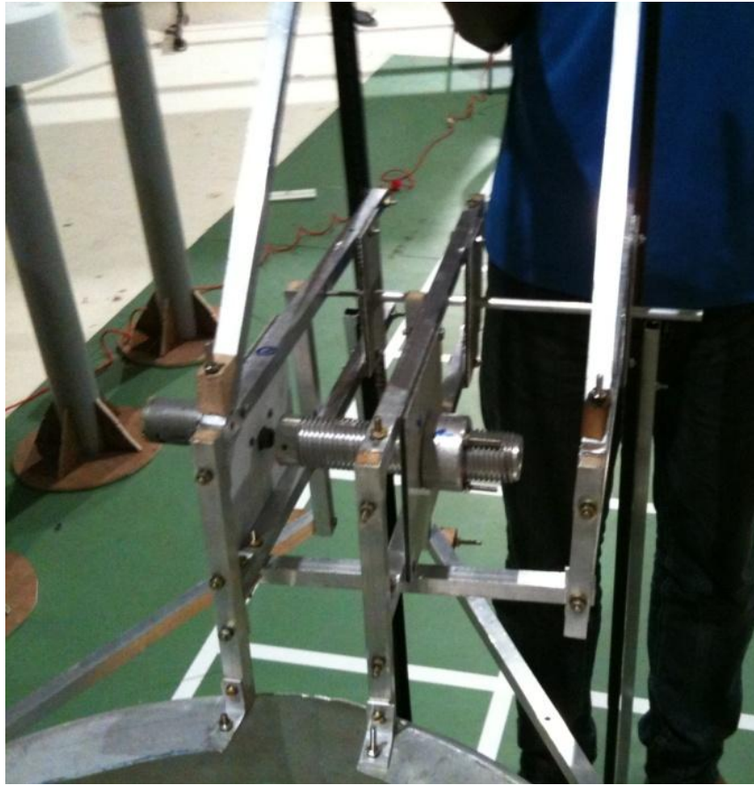
Screw clamp of the candle base mechanism
