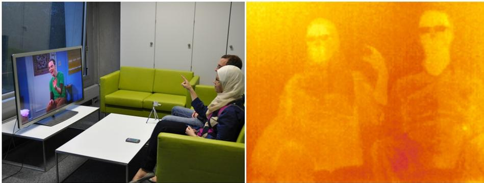
**Figure 7.1:** *A thermal camera facing a TV can monitor users sitting behind the camera through thermal reflection.*
